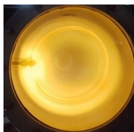
Discharge chamber, detector of millimetric radiation and focusing set-up in the Observatorio Astronómico de Yebes to study the rotational emissions of radicals and molecules generated in cold plasmas.
