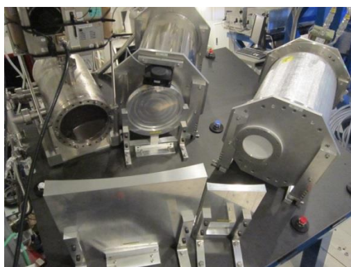
Discharge chamber, detector of millimetric radiation and focusing set-up in the Observatorio Astronómico de Yebes to study the rotational emissions of radicals and molecules generated in cold plasmas.
