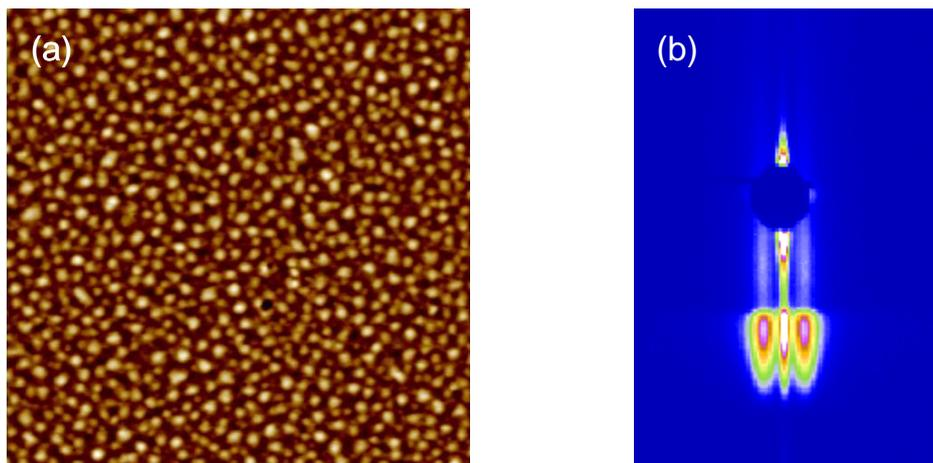
**Figure 1** (a)AFM tapping mode height image ( $5 \times 5 \mu\text{m}^2$ ) and (b) GISAXS pattern of a PBT film 13 nm thick.
