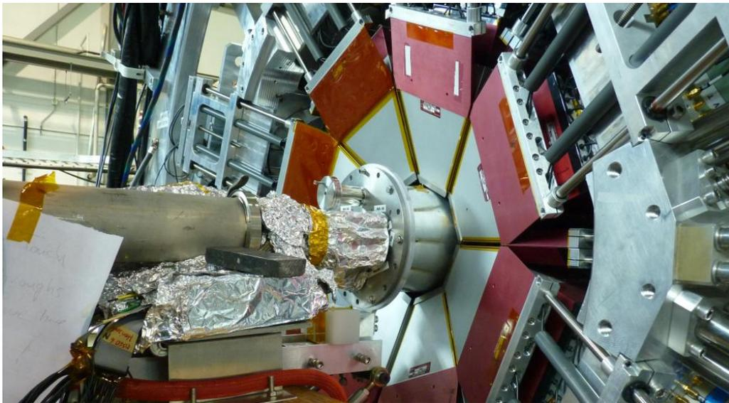
**Figure 3.10:** TIGRESS array closed around the reaction chamber. In this shot the eight clovers forming a ring at  $90^\circ$  can be seen. In particular, it is the BGO crystals surrounding each of the clovers that are visible.
