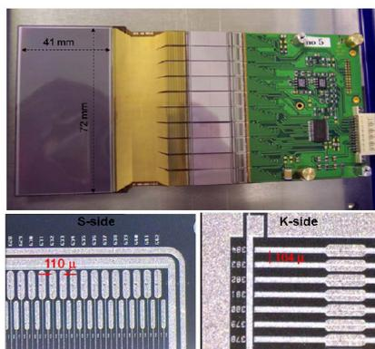
Figure 2.11: Photograph of a Micro-Strip Double Sided Silicon Detector (DSSD), showing the 0.3 mm thick sensor and with two pictures zoomed to the readout area, indicating the readout pitch which is  $110 \mu$  and  $104 \mu\text{m}$  for the S-side and K-side respectively. Image taken from [50].
