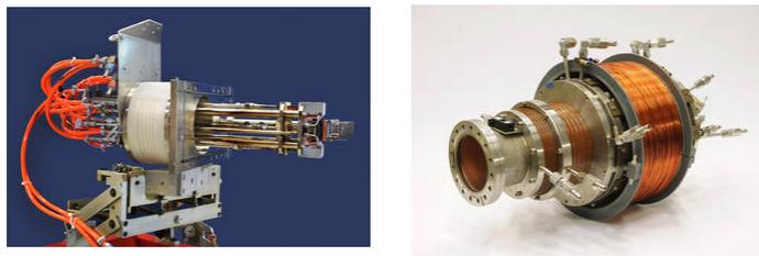
Figure 2.2: Pictures of the sources PIG(left) and MUCIS (right). From [57]
