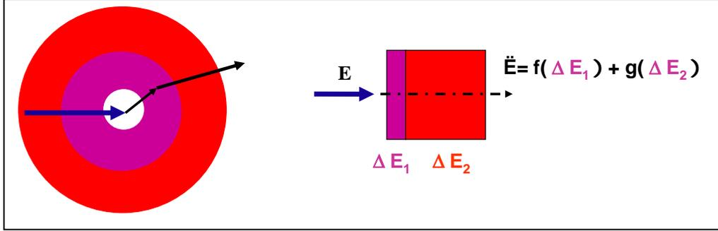
Figure 1: In the two layer detector approach, the estimated final energy is proportional to the energy deposited in each layer.
