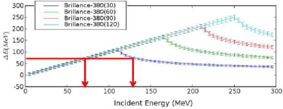
Figure 2: Deposited energy in different thickness layers of the Brilliance 380 scintillator,  $\text{LaBr}_3(\text{:Ce})$ , in function of the incident energy of the protons, following the Bethe-Bloch expression (1)
