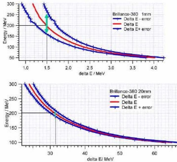
Figure 4: Incident energy vs. deposited energy in the 1 mm  $\text{LaBr}_3(\text{:Ce})$  and 20 mm  $\text{LaBr}_3(\text{:Ce})$  layers.
