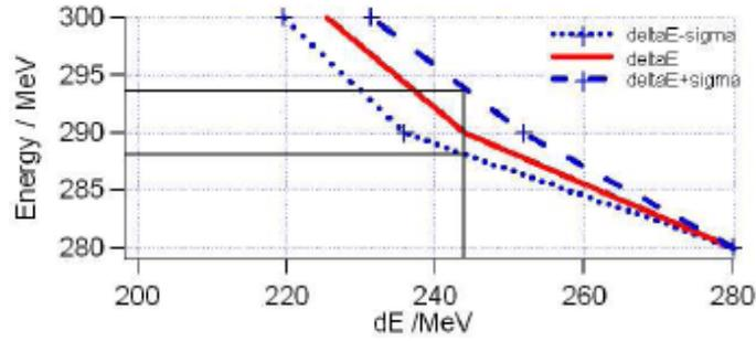
Figure 6: Incident energy vs. deposited energy in the 30 mm  $\text{LaBr}_3(\text{:Ce})$  and 150 mm  $\text{LaCl}_3(\text{:Ce})$  detector.
