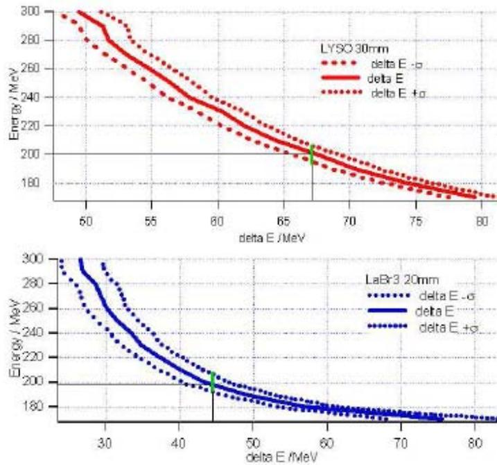
Figure 5: Incident energy vs. deposited energy in the 30 mm LYSO and 20 mm  $\text{LaBr}_3(\text{:Ce})$  layers.
