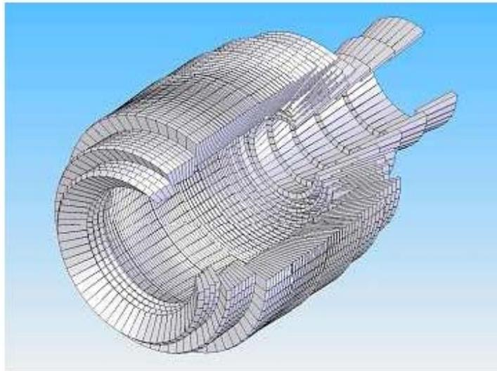
Figure 7: Shape of the calorimeter proposed by the Santiago de Compostela group.
