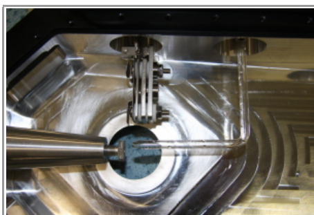
In the heart of the LOI88 experiment: this is the point where the metal ions (from the left) enter the drop.
