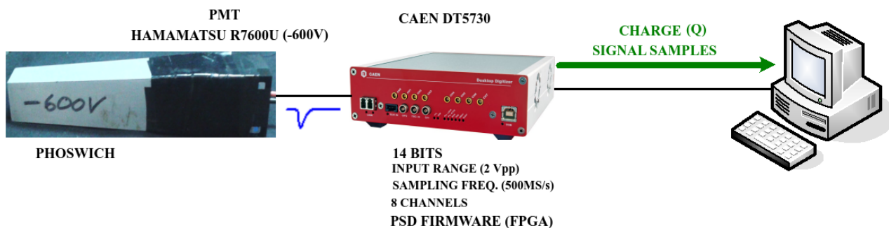
Figure 2. Digital Readout Electronic System.
