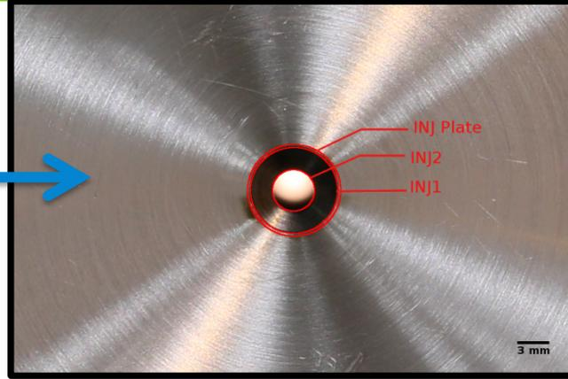
Results of the internal realignment for the injection and extraction electrodes to a precision of 0.1mm
