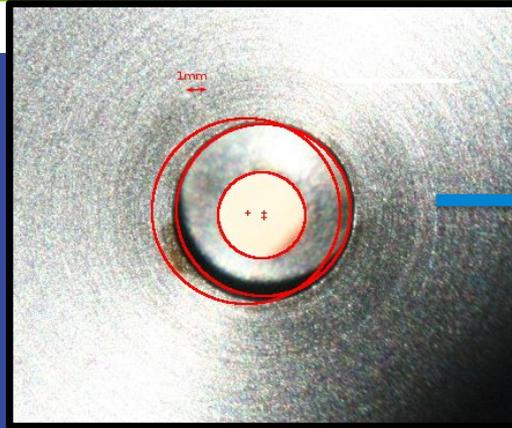
Measured misalignment of the injection (top) and extraction electrodes was 0.75mm
