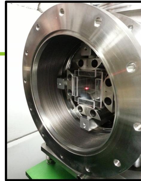
External alignment was done by aligning both sides of ISCOOL to the beamline quadrupole triplets, using a RILIS laser and the target
