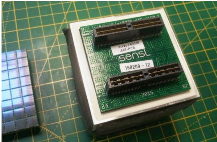
Fig. 1.1: SensL J-series array attached to the LaBr3 2"x2"x2" scintillator from Krakow
