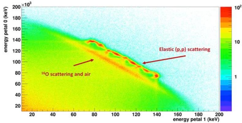
Fig. 2.6 First results from water target 500 um, 200 MeV protons.
