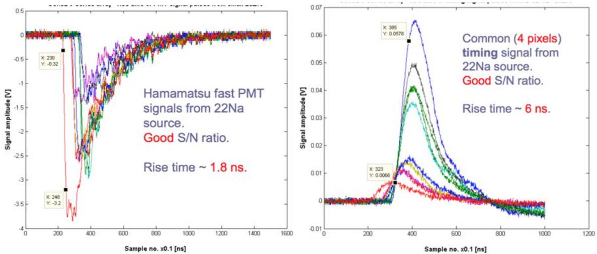
Fig 1.3: Comparison of timing output from Hamamatsu fast PMT and SensL J-series SiPM
