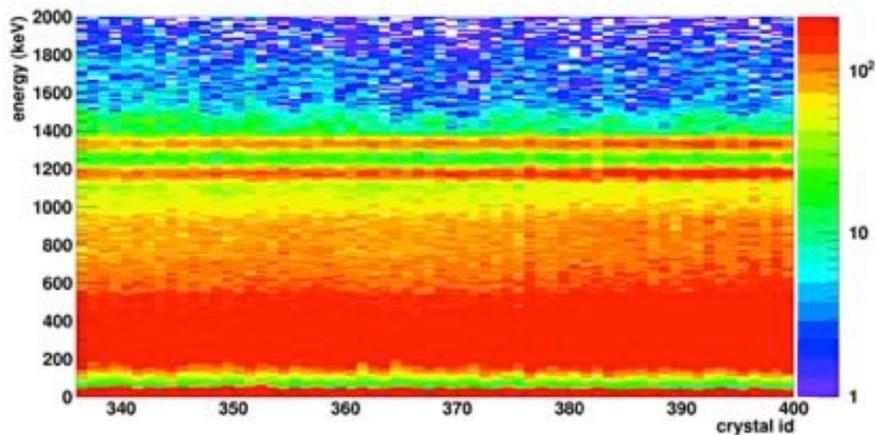
Fig. 2.4 Co-60 source calibration of one petal. All 64 crystals precisely calibrated.
