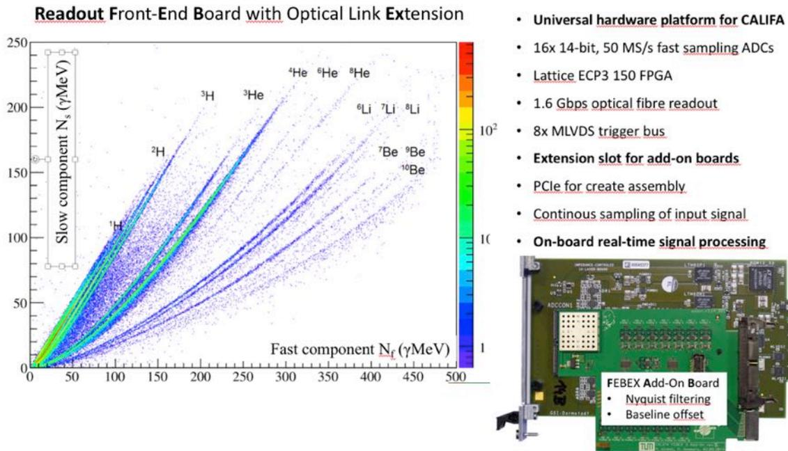
Fig. 2.9 Universal hardware readout-platform has been developed for the full CALIFA array.
