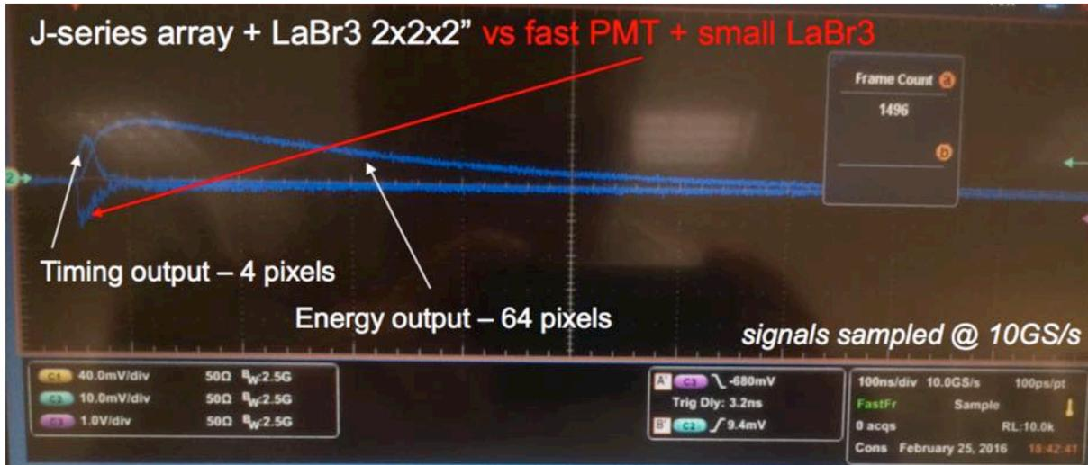
Fig. 1.2: SensL J-series array + LaBr3 2x2x2" vs fast PMT + small LaBr3
