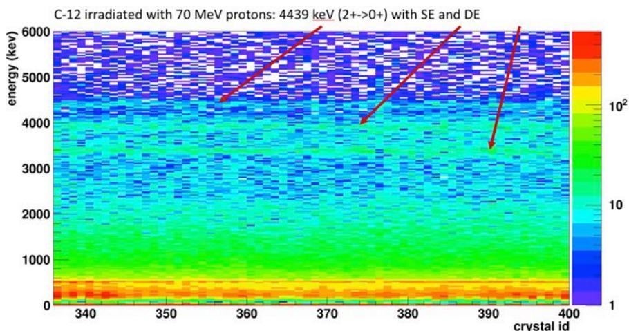
Fig. 2.5 Graphite block irradiated with 70 MeV protons to excite 2+ state at 4439 keV in  $^{12}\text{C}$ . Photo-peak, single and double escape peaks are visible. Also, the 511 keV visible.
