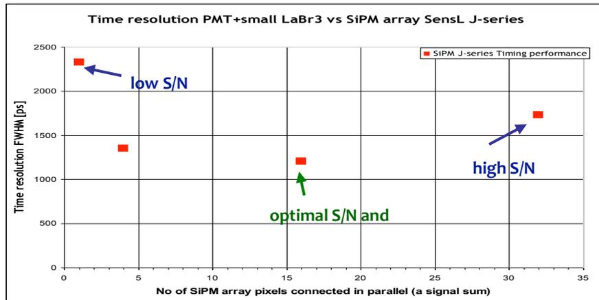
*Fig.4: Time resolution op PMT vs SiPM readout*
