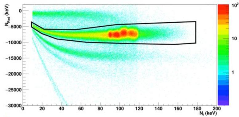
Fig. 2.8 A cut on the stopped proton band (inside black polygon) with 4 peaks from elastic scattered protons, cleans the events of all non-proton contributions.
