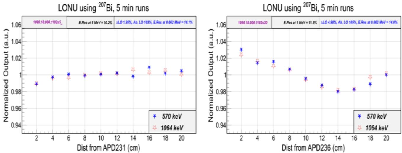
**Figure 4. Left: The LONU of an excellent crystal measured with the GENP-USC test bench. Right: A crystal yielding a sub-average LONU, the two peaks of  $^{207}\text{Bi}$  providing a self-confirmation of each measurement.**
