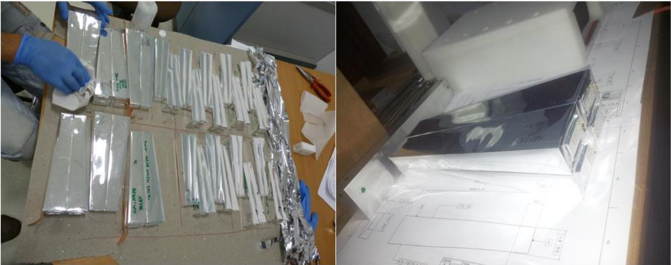
**Figure 1: Samples of the CsI(Tl) crystals being tested in this work.**
