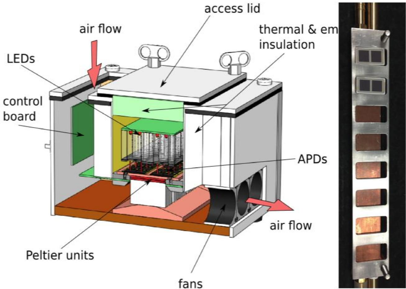
**Figure 2. Left: The IEM APD test bench, highlighting the different components required to characterise the resident APDs. Right: A row of APDs on the copper heat controlled backing.**
