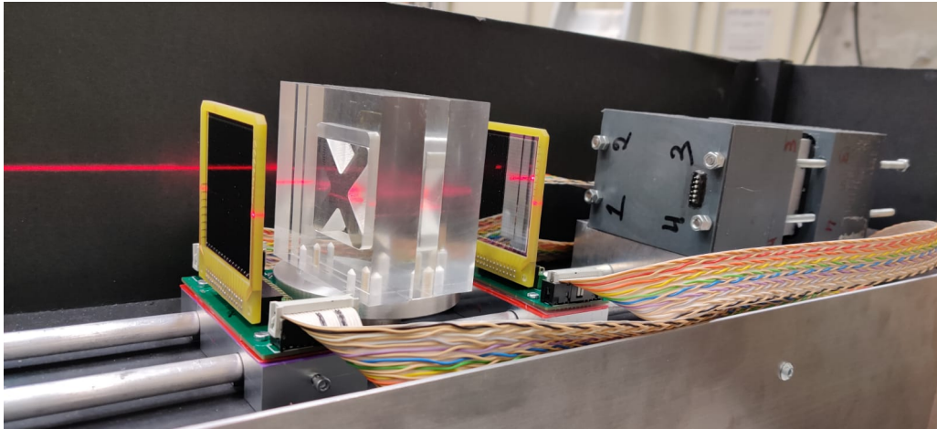
Figure 16: The experimental set up used at Centrum Cyklotronowe Bronowice (Kraków, Poland) June 4-7, 2021, not shown is the cover, as the Si detectors have to be in full darkness.
