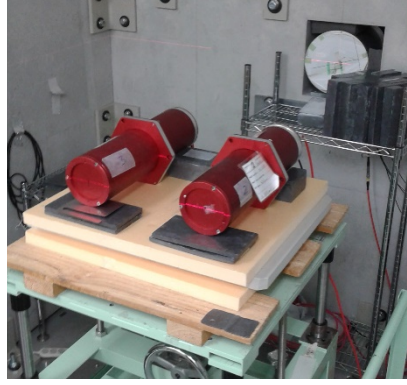
Fig. 1. A picture of the experimental setup. The \gamma -ray beam direction is indicated by the black arrow. The two \text{LaBr}_3\text{:Ce} detectors can be moved left-right to intercept the beam
