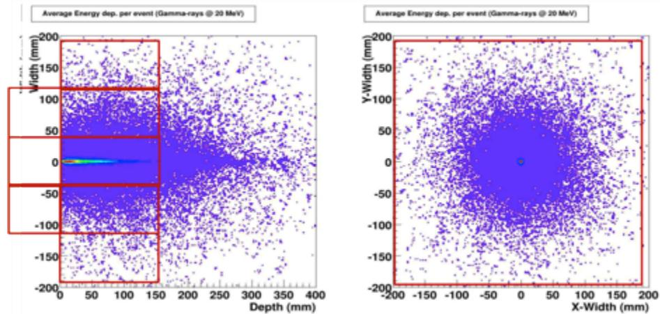
Gamma radiation average energy deposit per event inside an infinite volume of LaBr detector
