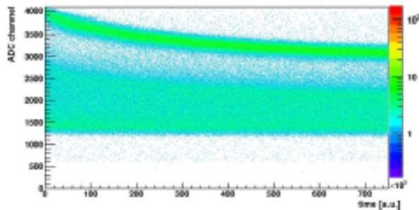
Gain gradient due to continuous heating
