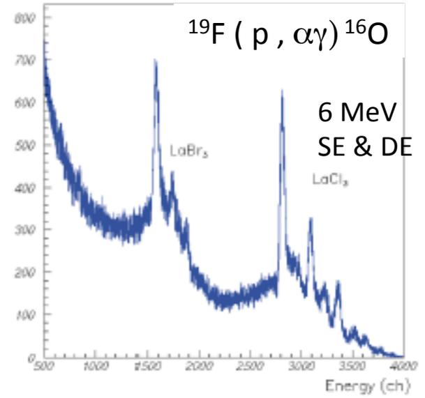
The resolution for the LaBr<sub>3</sub>(Ce) response in the phoswich compared to an individual crystal. As seen the phoswich conguration does not deteriorate the resolution. The high energy points where taken shooting 1 MeV p on Teflon.
