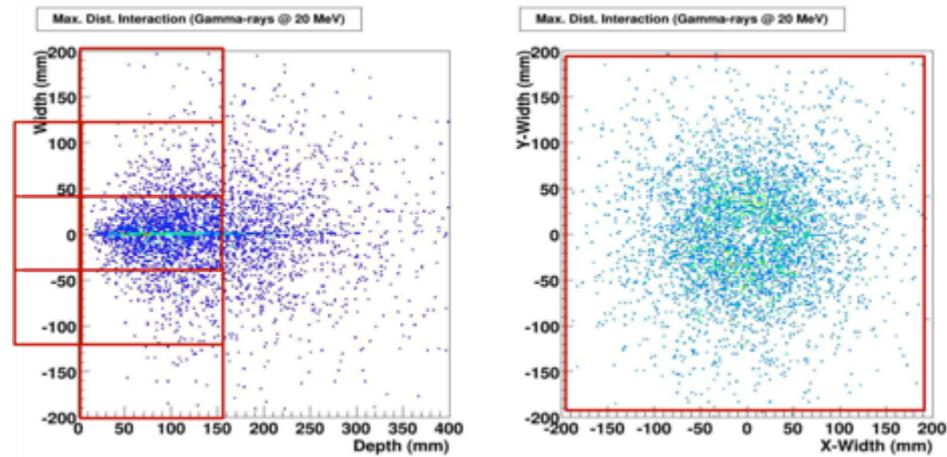
Maximum distance between interactions - absorbing one incident gamma inside a crystal  $10 \times 10 \times 150 \text{ mm}^3$
