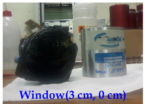
A detailed scan with a grid of 0.5 cm was performed using the 662 keV gamma rays of a <sup>137</sup>Cs collimated source.
