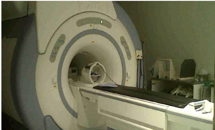
Figure 6: The 3-T MRI magnet at the York Neuroimaging Centre. The detectors are placed on the side of circular cage shown in the centre of the magnet. The cables from the detectors can be seen stretching along the bed.
